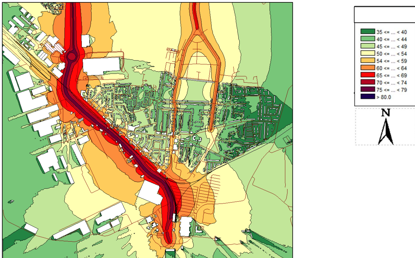
Diagram 15.1.3: Baseline CadnaA acoustic noise model, illustrating the existing L_{A10} noise climate around the Essex Project Site
